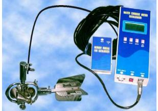
This Digital Water Current Meter is used to measure Velocity of water flow directly in m/s. The stainless steel spindle carrying the cup wheel freely rotates in the bearing assembly. The magnet and reed switch assembly produces one pulse per rotation. The rotation of the Water Current Meter is sensed by sensor & gives pulsed output signal.
